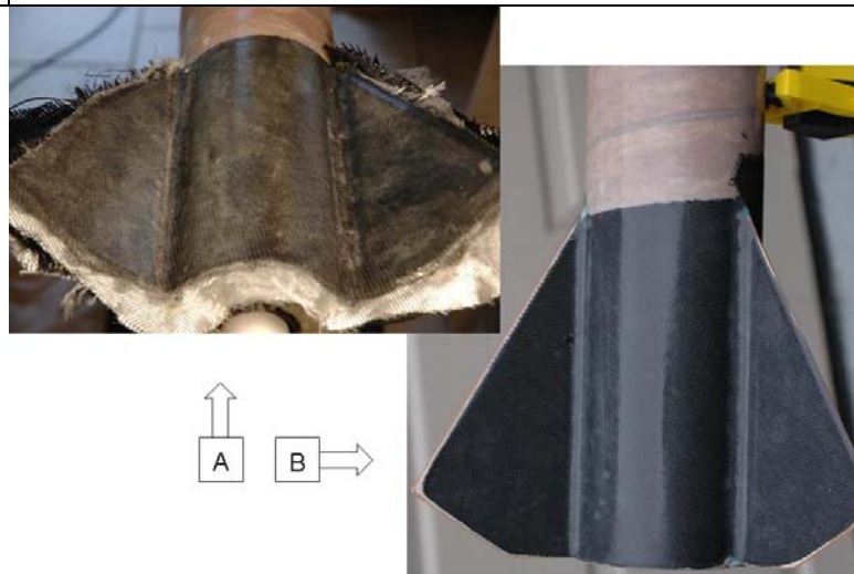
(A) Fins with 1 layer 6 oz. Carbon Fiber covered by 1 layer 10 oz Fiberglass (B) Fins after epoxy cures and surface is sanded (surface is wet for sheen)
