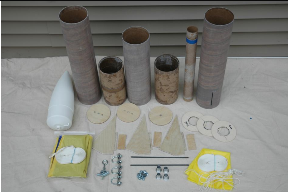
All parts in the kit ready to build after fiberglassing Body Tubes, Couplers, Fins and Bulkplates (Couplers are fully assembled in this photo).
